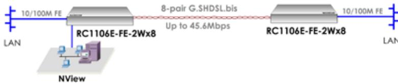
Delivering Fast Ethernet services over 16 wire copper cables
