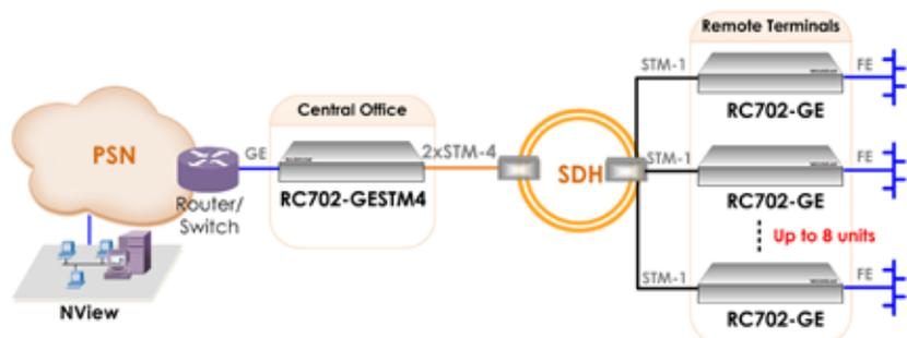
Aggregates 8 Fast Ethernet to Gigabit Ethernet over two STM-4 links
